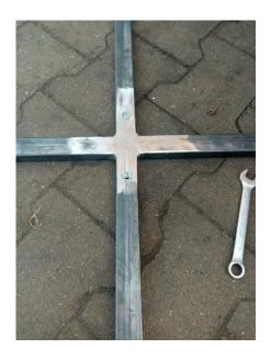
Set the cross base of the construction on a stable surface
